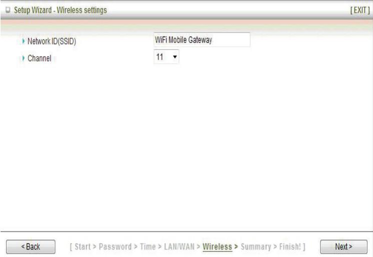
The screenshot shows the 'Setup Wizard - Wireless settings' window. It has a title bar with a close button and '[EXIT]'. The main area contains two fields: 'Network ID(SSID)' with the value 'WiFi Mobile Gateway' and 'Channel' with a dropdown menu set to '11'. At the bottom, there is a '< Back' button, a breadcrumb trail '[ Start > Password > Time > LAN/WAN > Wireless > Summary > Finish! ]', and a 'Next >' button.
